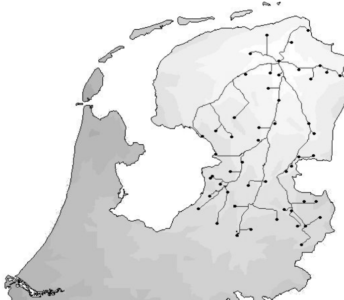
Figure 6: The routes calculated to and from Groningen. The background shading reflects the overall cost of the trip, where darker grey means a more expensive trip.
